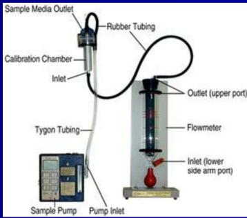
Active sampling – Calibration of Flow Rate (Cont'd)
