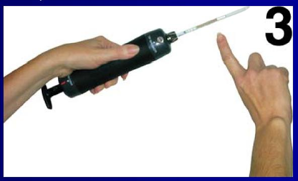
Colorimetric Devices – Indicator Tube (passive)
