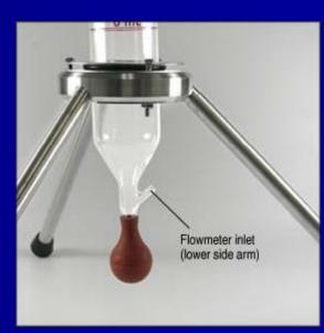
Active sampling – Flow Rate Measurements
